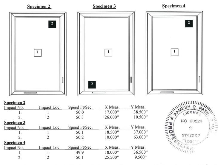
Results: All specimens tested resisted the large missile impact, without penetration of the inner plane of the glazing. With no tear forming longer than 5" or no opening through which a 3" diameter solid sphere could freely pass.
