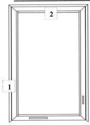
Deflection / Permanent Set were measured with two (2) Mitutoyo dial indicators SN- mky019, and SN - mtj695 Measurements were taken at:
